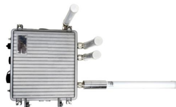
LoRawan outdoor base station
