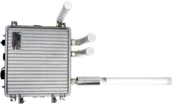
LoRawan outdoor base station
