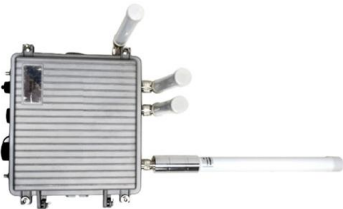
LoRawan outdoor base station
