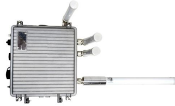
LoRawan outdoor base station
