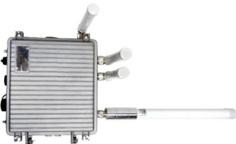
LoRawan outdoor base station
